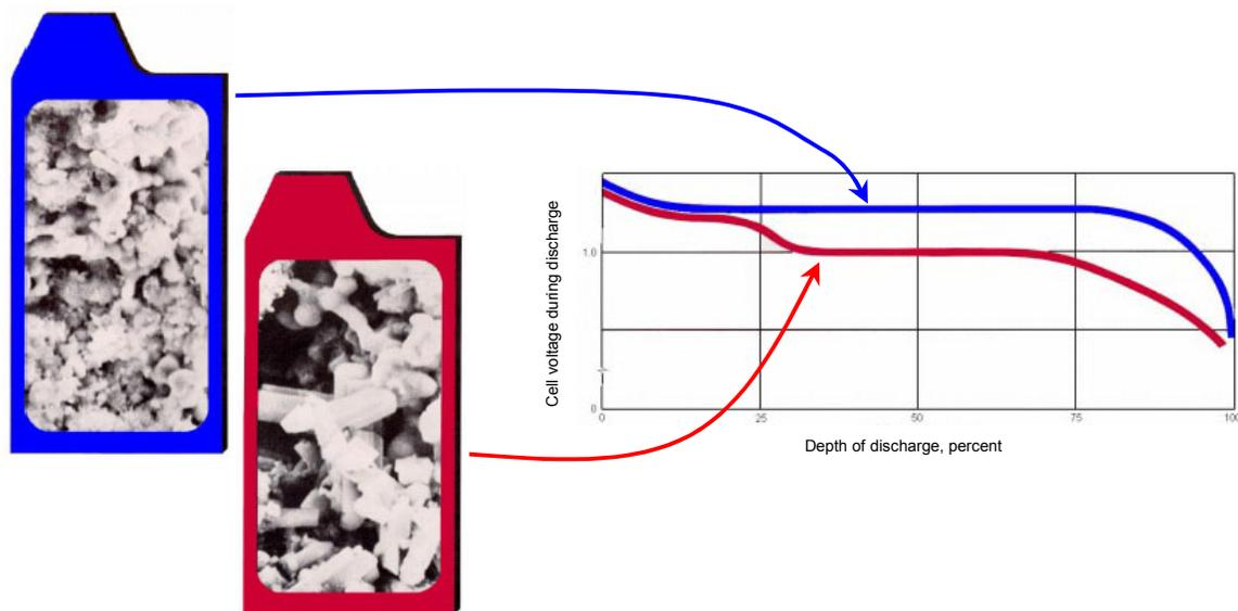
**Figure 1 – Normal (top) and ‘memorized’ (bottom) Ni-Cd cells (from Pensabene & Gould<sup>2</sup>)**
