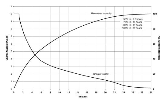
Fig. 3 - Charge characteristic of a 48 V 80 Ah SMC battery
