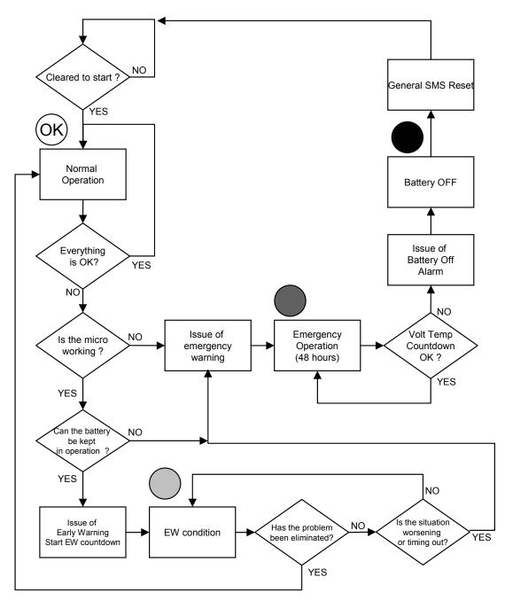
Fig. 5 Flowchart of main loop of the battery management system with sequence of operations in case of failures.
