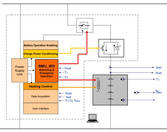
Fig. 4 - Block Diagram of the SMS for SMC battery.
