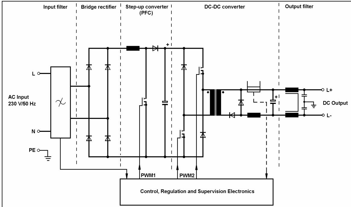
Figure 4 Rectifier Stage
