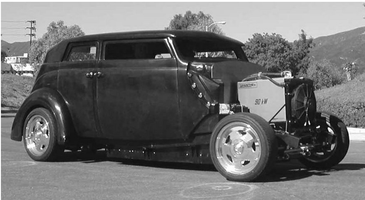
Figure 2. Electric Vehicle with 90KW AC Motor Controller and 6.6KW Integrated Charger 2
