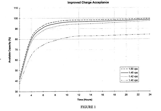
Most telecom plants require a slightly higher end voltage; in some cases 43.75 volts is specified (Bellcore TA-NWT-000406). This corresponds to 1.82 volts per cell for a lead acid battery and 1.15 volts per cell for a nickel cadmium battery. In both cases, it means that a little less than full capacity can be utilized. In other words, the discharge performance of the ANC telecom battery should be expected to be very similar to that of a VRLA battery.
