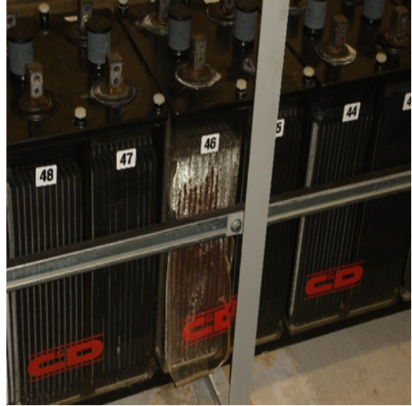
Figure 2. Ruptured cell, cause unknown, side is still attached to the cover, no parts ejected, no violence displayed, parts intact but separated
