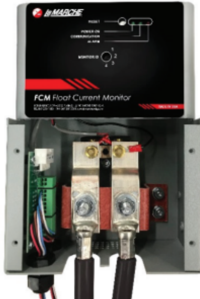
Figure 6. Float current monitor that works in conjunction with a battery charger. To install this the circuit needs to be interrupted so that this can be installed in one of the cable circuits that goes from the battery to the charger. The current value is relayed to a monitor or alarm relay.
