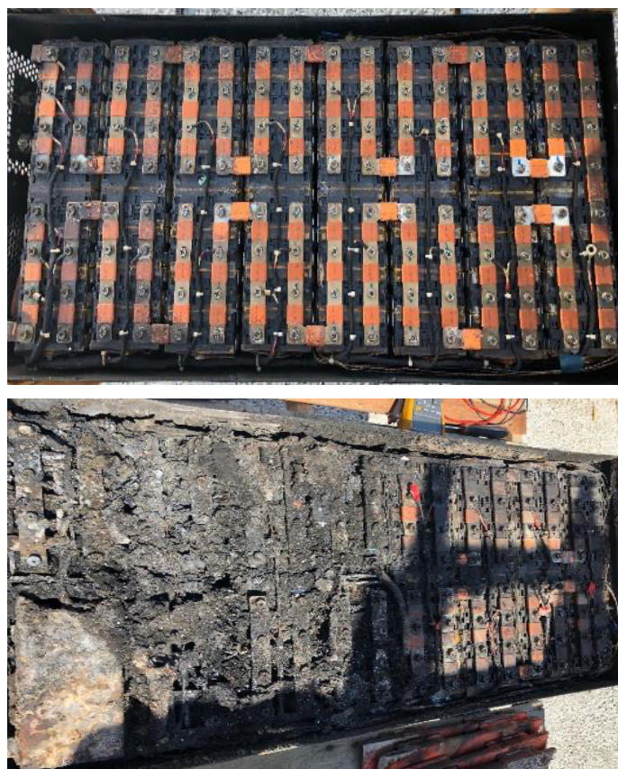
Figure 7. Results of water FSS test, showing initiating module (bottom) and module immediately above (top)
