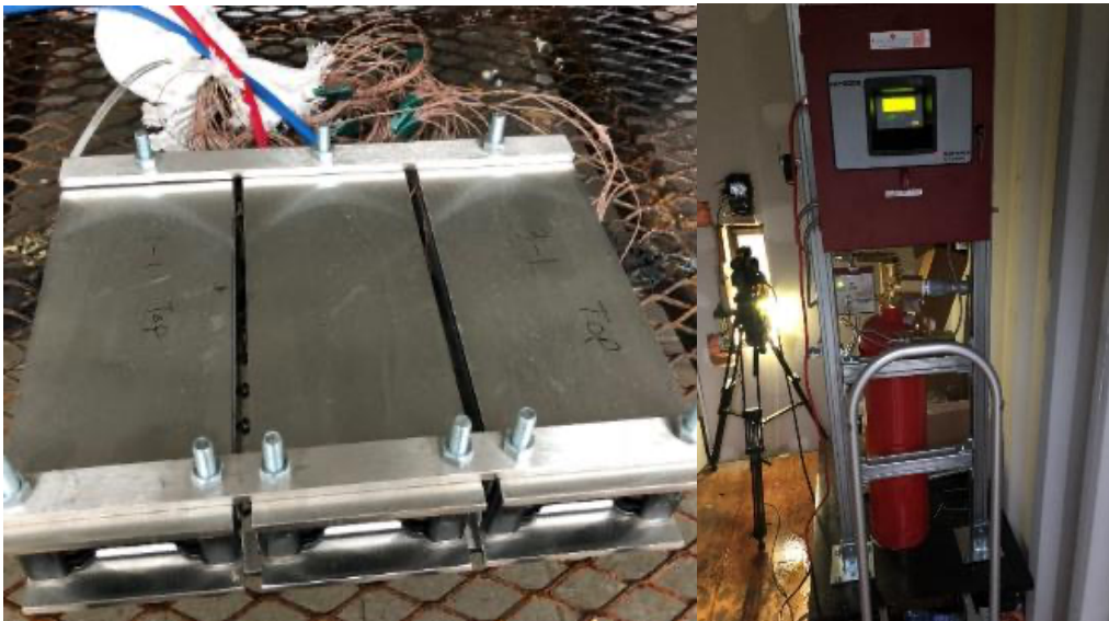
Figure 3. Test setup with three cell blocks and Novec FSS
