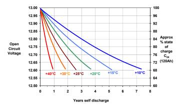
Figure 2 – Self Discharge Characteristics of TPPL
