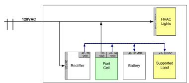
Figure 1 – Typical Fuel Cell System Configuration
