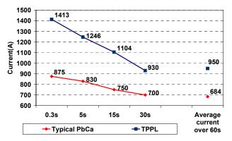
Figure 3 – High Rate Performance of TPPL
