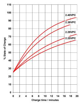
**Figure 5 – Recharge Characteristics of TPPL**
