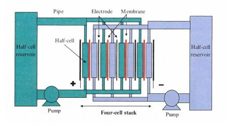
Figure 1. Concept of the Redox Flow Battery System
