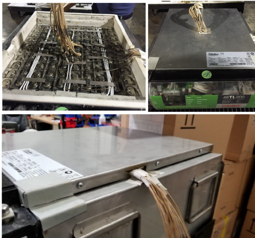
Figure 4. Sodium nickel chloride Module level test unit with instrumentation modification
