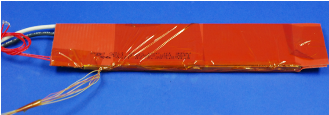
Figure 3 Thermal Technique using Externally Powered Heaters
